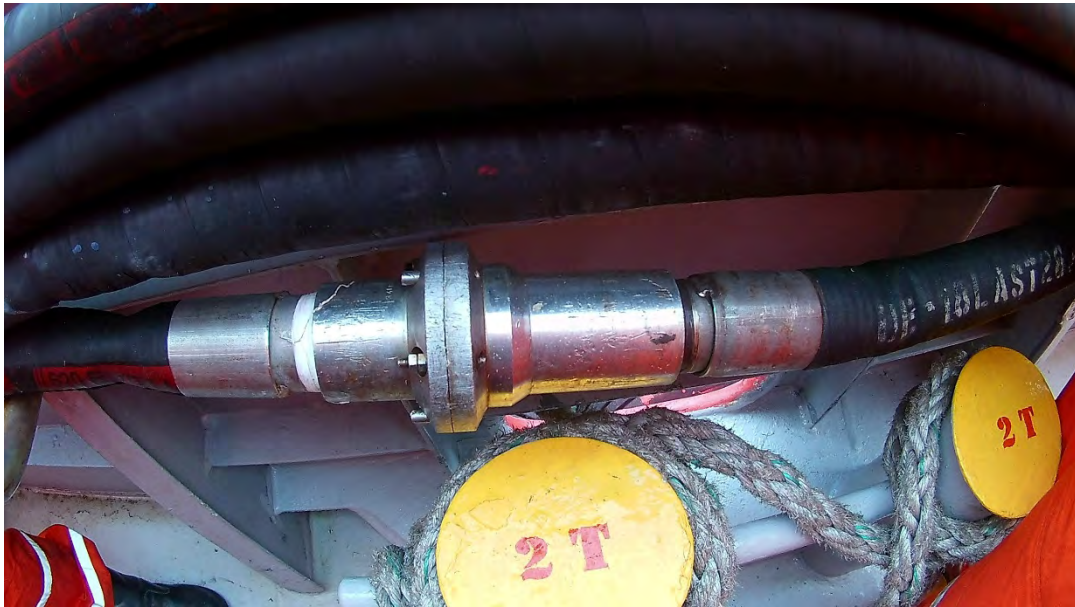
PHOTOGRAPH 33 MARINE BREAKAWAY COUPLING.
