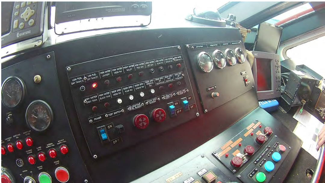
PHOTOGRAPH 11 BILGE ALARM AND WATERTIGHT DOOR CONTROL PANEL (TESTING).
