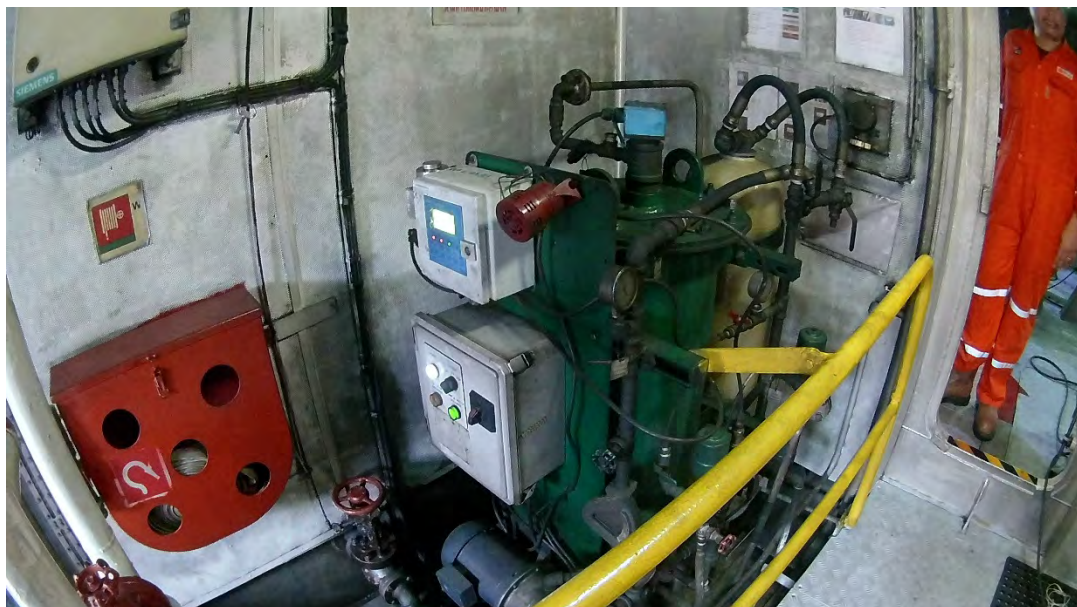
PHOTOGRAPH 58 OILY WATER SEPARATOR TESTING.
